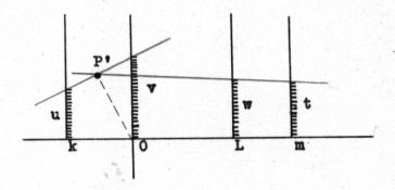
The points marked u, v, w, and t are then (k, u), (0, v), (L, w), and (m, t) respectively. The co-ordinates of P' may then be found and we write the equation of the line through P' and the point (m, t). In this equation we replace x and y by L and w and we have as the equation represented by this nomogram
