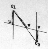
$\frac{f_1}{f_2} = \frac{f_3}{f_4}$  may be represented by two parallel supports each carrying two scales and having origins on a transversal. The index is two straight lines intersecting on the transversal.
