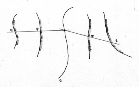
In this case we recognize the so called double alignment chart. The theory of such charts has been worked out by studying the two charts of which it is composed. Charts which do not result from this consideration can be devised by simply choosing methods of combining two indices.
